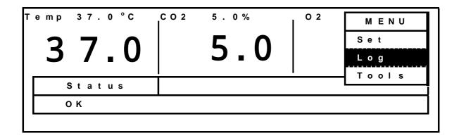
**2.** The log will be displayed with dots. Press the Up Cursor Key and Down Cursor Key to switch between the temperature,  $CO_2$  density and  $O_2$  density displays. Press the Left Cursor Key and Right Cursor Key to scroll the displayed data (Left Cursor Key: older data, Right Cursor Key: newer data).
